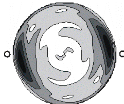
Fig. 10. Contour plot of u_\theta in plasma cross-section (flank circles show the positions of antenna legs)
