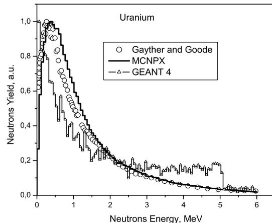
Fig.10. Neutron spectra for Uranium target
