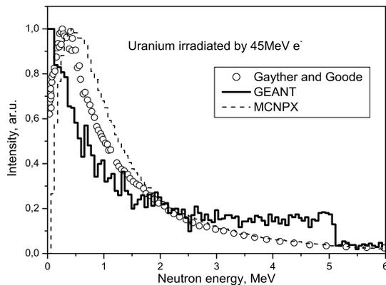
**Fig.3.** Neutron spectra simulation and experimental data of Uranium irradiated by 45 MeV electrons
