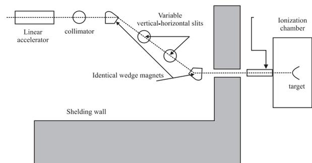
**Fig.1.** Scheme of the experiment by W.C. Barber and W.D. Georget
