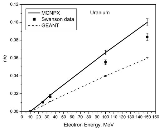
Fig.7. Neutron yield for Uranium target versus initial electron energies
