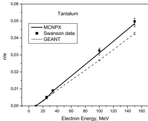
Fig.8. Neutron yield for lead Tantalum versus initial electron energies
