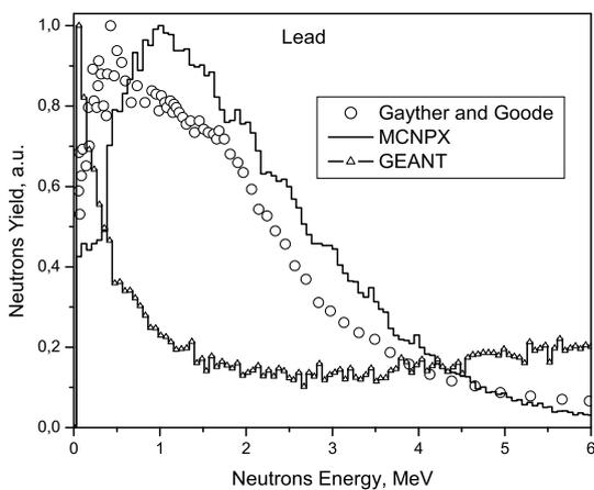
**Fig.11.** Neutron spectra for Lead target
