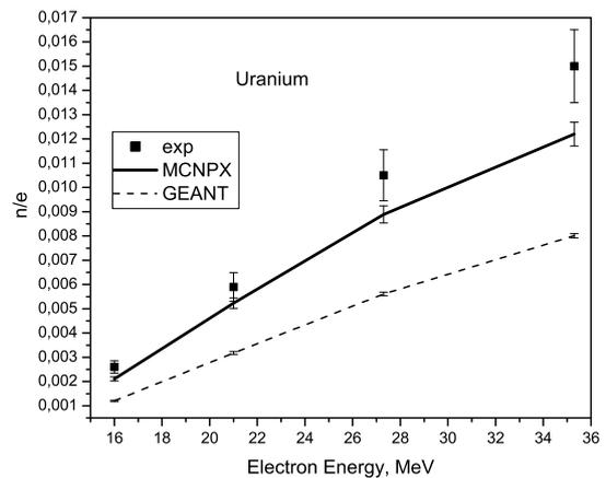
**Fig.4.** Neutron yields versus beam energy for Uranium target
