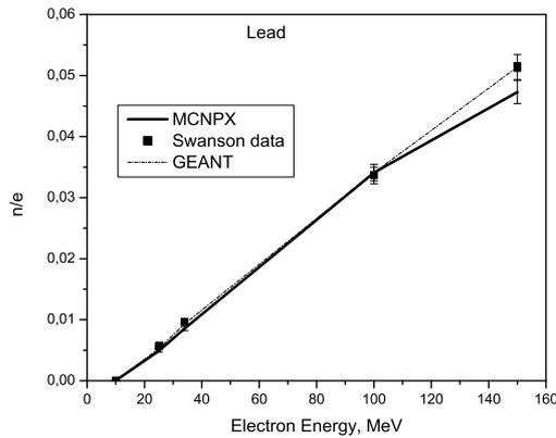
Fig.6. Neutron yield for lead target versus initial electron energies
