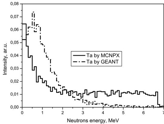
**Fig.2.** Neutron spectra simulation of Tantalum irradiated by 34 MeV electrons
