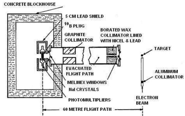
Fig.9. Experimental arrangement by D.B. Gayther and P.D. Goode
