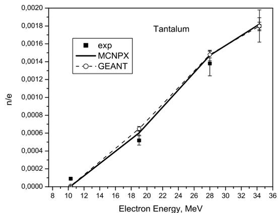
**Fig.5.** Neutron yields versus beam energy for Tantalum target
