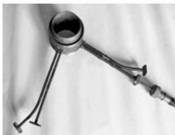
Fig. 2. Open barrel-shaped resonator
