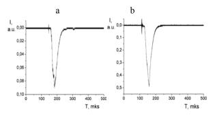
Fig. 4. Dependence of the optical radiation intensity on time for the wavelength 485 nm within a duration of one high-voltage pulse for gas pressures of P = 28 (a) and 4.8 Pa (b)
