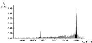
Fig. 3. The emission spectra of discharges in air at a pressure P = 4.8 Pa
