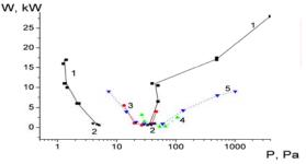
Fig. 1. Dependences for breakdown power of a microwave signals with a stochastically jumping phase versus a pressure for air in the optimal BPG mode (curves 1 - 1, 2 - 1), in the non-optimal BPG mode:
