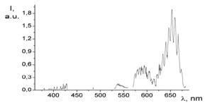
Fig. 2. The emission spectra of discharges in air at a pressure P = 28 Pa
