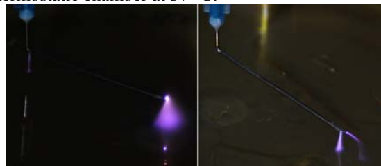
Fig. 2: Negative (left) and positive (right) corona discharge. The parasite discharge at the elbow for 90° bent needle (left) and discharge at the needle edges for 80° bent needle (right)
