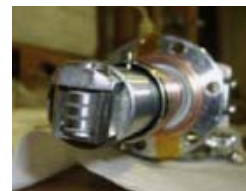
Fig. 1. New version of the 4-channel probe with AlN radiators of 10 mm in dia. and 2 mm in thickness [5]
