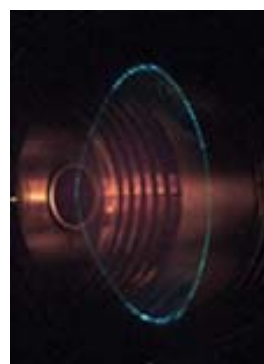
Fig. 3. Example of defining the last closed magnetic surface measurements on the hurricane-2M torsatron: mode K\varphi=0.295 ; B_0=0.1 T; \langle B_{\perp}/B_0 \rangle \approx 1.5\% ( I_{corr} \approx 100 A); average radius \bar{a} \approx 17.3 cm; \Delta_{axis} \approx 5.9
