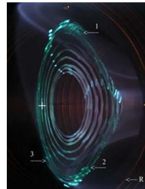
Fig. 3. Magnetic surface structure at the configuration mode with  $k_\varphi = 0.31$  and  $\langle B_\perp/B_0 \rangle = 1.14\%$ : the mean radius of the closed magnetic surface, which is adjacent to three whiskers (1, 2, 3), i.e., remains of the broken magnetic islands with  $i/2\pi = 1/3$ , is  $a \approx 17.3$  cm;  $\Delta \approx 9$  cm
