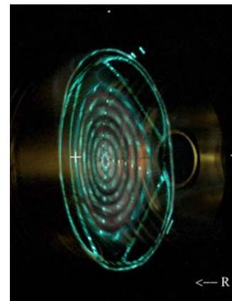
Fig. 4. Magnetic surface structure at the configuration mode with  $k_\varphi = 0.32$  and  $\langle B_\perp/B_0 \rangle = 1.58\%$ : the mean radius of the closed magnetic surface, which is adjacent to the chain of magnetic islands with  $i/2\pi = 1/3$ , is  $a \approx 17$  cm;  $\Delta \approx 6.65$  cm;  $\delta \approx 2.5 \dots 5$  cm; island lengths are  $l_{is} \approx 20.6, 21$  and  $41$  cm; the mean radius of the island centers (O-points) is  $r \approx 13$  cm
