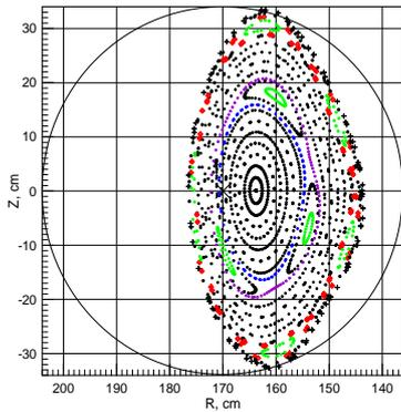
Fig. 10. Magnetic surface structure at the configuration mode with  $k_\phi=0.31$  and  $\langle B_\perp/B_0 \rangle=1.5\%$ : the mean radius of the closed magnetic surface, which is adjacent to a chain of magnetic islands with  $i/2\pi=2/5$ , is  $a \approx 20$  cm;  $\Delta = -6.26$  cm;  $i/2\pi(0) \approx 0.25$ ;  $i/2\pi(a) \approx 2/5$
