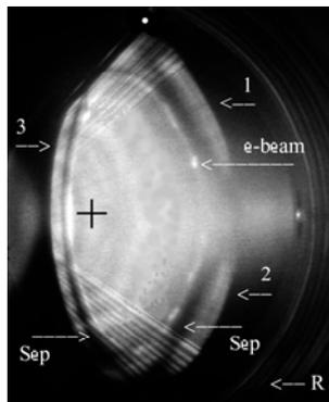
Fig. 1. Visual demonstration of the island divertor operation. The view of the low-density plasma confinement region in the Uragan-2M torsatron: mode  $k_\varphi \approx 0.295$ ,  $\langle B_\perp/B_0 \rangle \approx 1.8\%$ ; mean radius of the last closed magnetic surface  $a \approx 16.3$  cm; thickness of separatrix region  $Sep \approx 0.45 \dots 2.5$  cm; transverse dimensions of islands  $\delta \approx 2.3 \dots 4.7$  cm; mean radius of O- and X-points of islands  $r \approx 19.6$  cm
