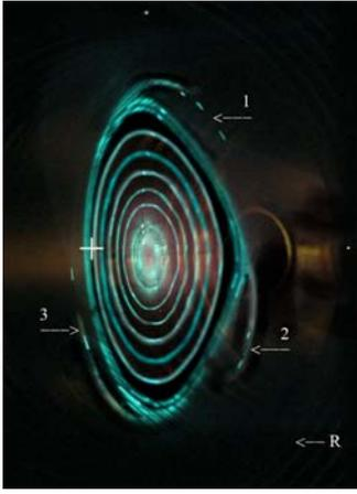
Fig. 5. Magnetic surface structure at the configuration mode with  $k_\phi=0.32$  and  $\langle B_\perp/B_0 \rangle=1.34\%$ : the mean radius of the closed magnetic surface, which is adjacent to three whiskers (1, 2, 3), i.e., remains of the broken magnetic islands with  $i/2\pi=1/3$ , is  $a\approx 14.4$  cm;  $\Delta\approx 7.7$  cm
