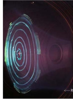
Fig. 8. Magnetic surface structure at the configuration mode with  $k_\phi=0.295$  and  $\langle B_\perp/B_0 \rangle=3.21\%$ : the mean radius of the closed magnetic surface, which is adjacent to a chain of five magnetic islands with  $i/2\pi=2/5$ , is  $a\approx 16.8$  cm;  $\Delta\approx 1.0$  cm
