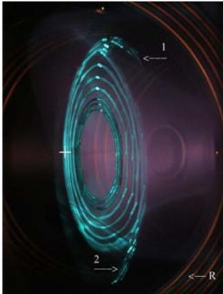
Fig. 7. Magnetic surface structure at the configuration mode with  $k_\phi=0.36$  and  $\langle B_\perp/B_0 \rangle=2.03\%$ : the mean radius of the closed magnetic surface, which is adjacent to two whiskers (1, 2), i.e., remains of two magnetic islands with  $i/2\pi=1/2$ , is  $a\approx 14.3$  cm;  $\Delta\approx 7.6$  cm
