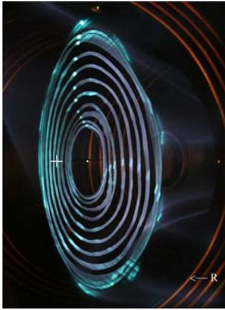
Fig. 6. Magnetic surface structure at the configuration mode with  $k_\phi=0.33$  and  $\langle B_\perp/B_0 \rangle=1.92\%$ : the mean radius of the closed magnetic surface, which is adjacent to two neighboring chains of magnetic islands with  $i/2\pi=2/5$  and  $i/2\pi=3/7$ , is  $a\approx 19$  cm;  $\Delta\approx 6.4$  cm
