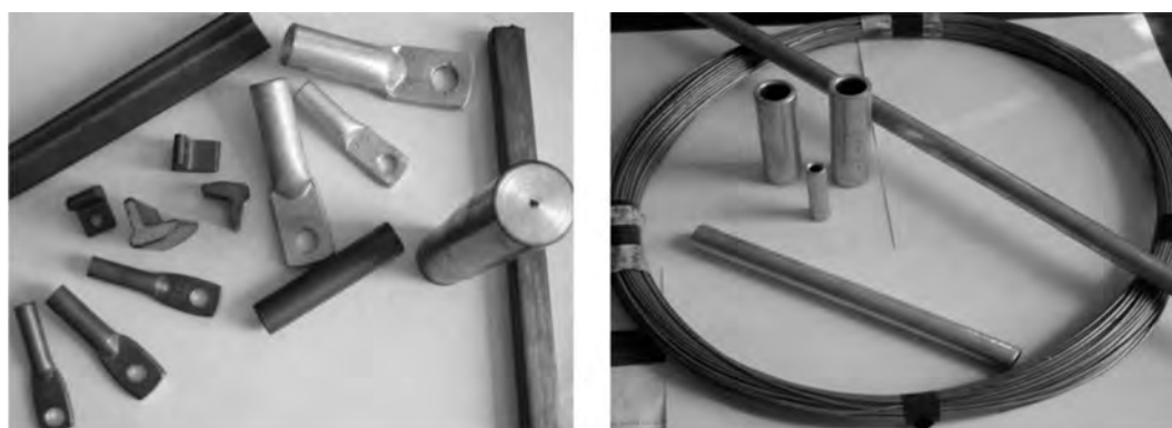
Fig. 25. Final products from recycled non-ferrous metals manufactured by TE processing and following extrusion
