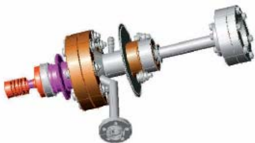
Fig. 2. Fundamental harmonic THz range demountable gyrotron with pulsed solenoid
