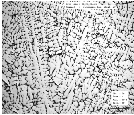
Fig. 1. AlCu4MgMn alloy microstructure before homogenization; enl: \times 100 .
