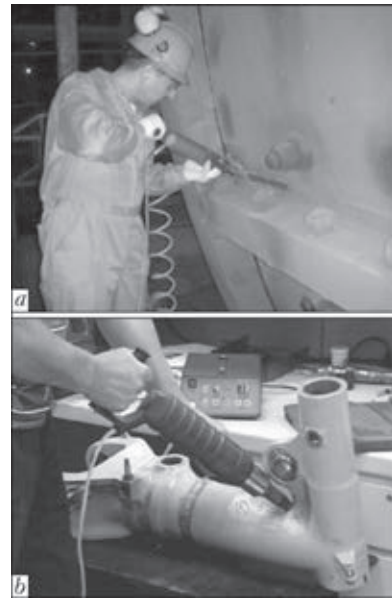
Figure 8. Examples of application of the UltraPeen system for fatigue improvement: a — of grinding mill when over 250 meters of welds were treated, b — of landing gear where critical from the fatigue point of view zone was treated
