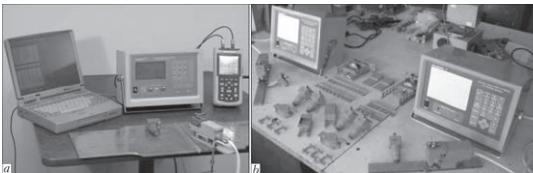
Figure 1. Ultrasonic Computerized Complex for residual and applied stress measurement: a — UltraMARS® model shown with a laptop and an oscilloscope; b — Next generation UltraMARS®-7 model shown with all transducers, transducer holders and attachments
