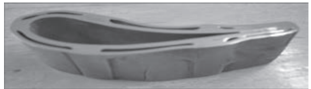
Figure 10. Turbine blade with complicated inner cooling gas channeling to be fabricated by additive manufacturing using electron beam physical vapor deposition (EB-PVD)
